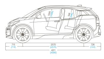
All dimensions in the technical drawings are given in millimetres. Luggage compartment volume 260–1,100 litres. The height of the BMW i3 with roof fin is 1598 mm. The height of the BMW i3 with roof fin is 1598 mm. The height of the BMW i3 with roof fin is 1590 mm. Provisional figures; any missing figures were unavailable at the time of publication.
